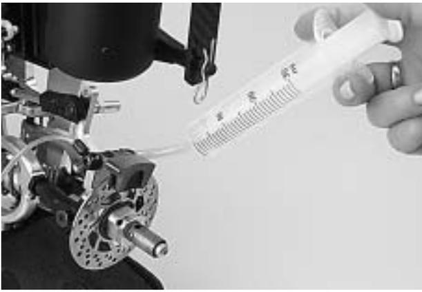
Press the injection with filling hose on the valve.
